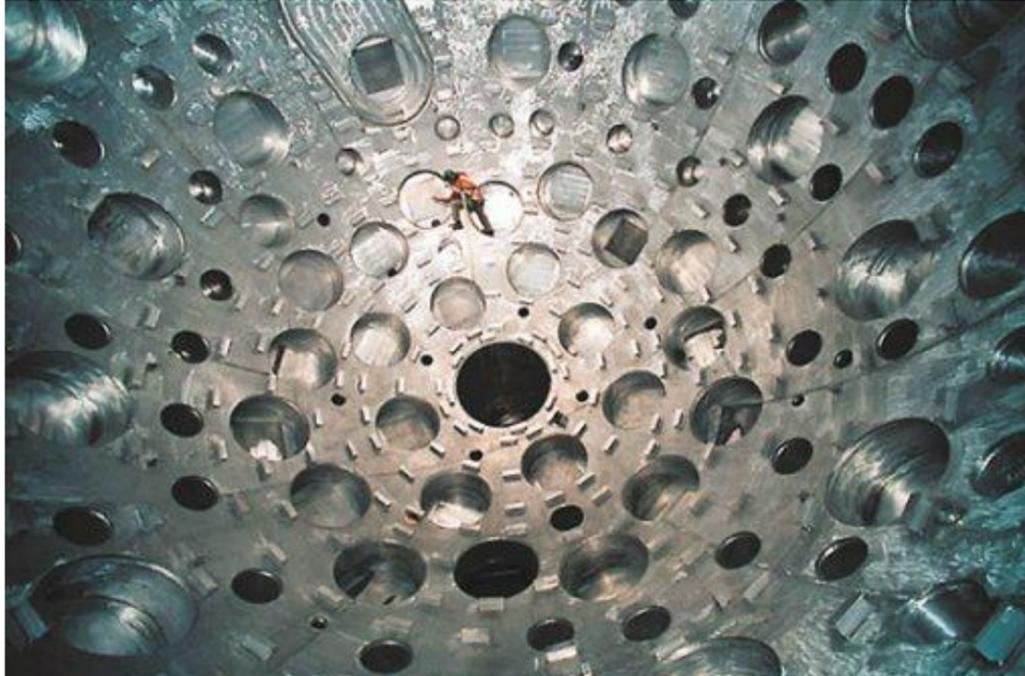
Inertial Confinement (Laser) Fusion (NIF) Target Chamber
